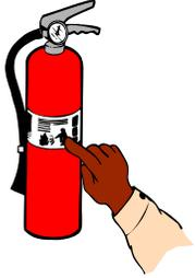
The letters on the label of an extinguisher indicate what type of fire to use it on (see below). Make sure to use the right extinguisher for the type of fire.
